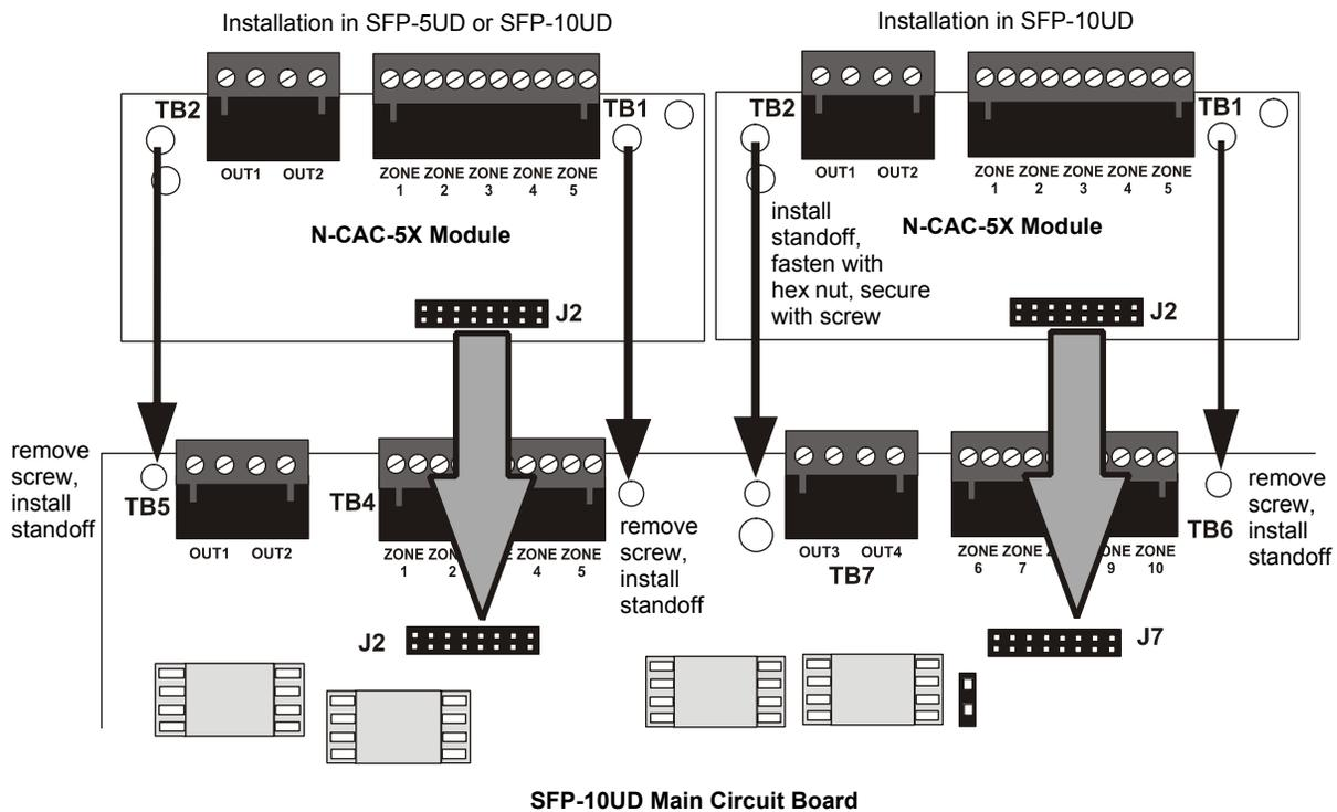
Figure 2.14 N-CAC-5X Module Installation
