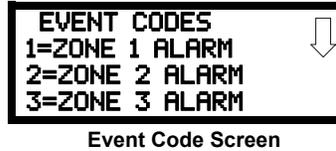
Pressing the down arrow key allows viewing of all Events associated with the selected Communication Format. Pressing the number corresponding to the event displayed in each screen will display its default active and restoral event codes which can be customized by the programmer.
