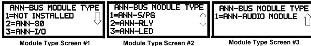
Press the number corresponding to the module type, if any, that is installed with the selected address. *This will enable the module.*
