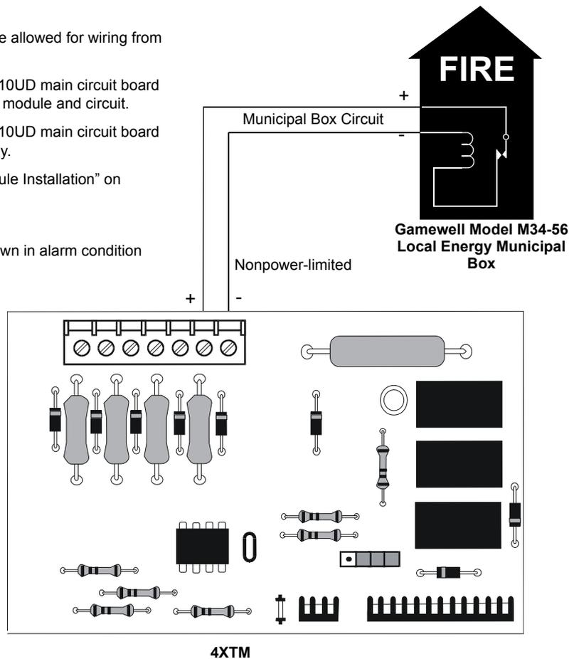
**Figure B.2 Municipal Box Connected to 4XTM Transmitter Module**
