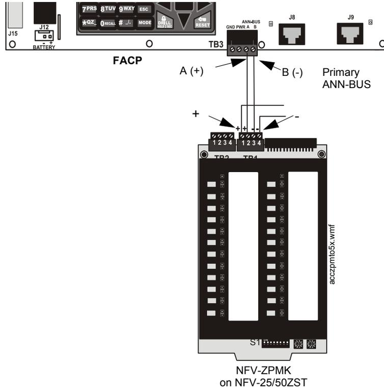
Figure 2.30 FACP Connection to NFV-25/50ZS/T Audio Panel
