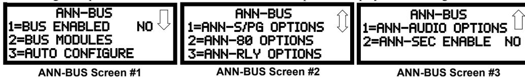
A variety of ANN-BUS option modules can be installed in the FACP. These devices communicate with the FACP over the ANN-BUS terminals on the control panel.
