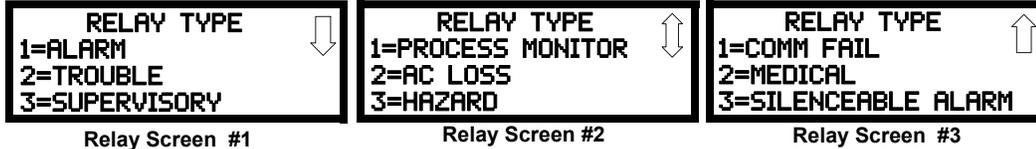
While viewing the selected screen, press the number corresponding to the desired relay type to program the main circuit board relay. The choice will be stored in memory and the display will return to the Relay Type Screen which will show the programmed type choice. Press the Escape key to return to the Relays Selection Screen and repeat the preceding procedure for the remaining relays.
