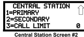
Central Station Screen #1 indicates whether the Central Station Reporting is enabled or disabled and if the Reports will be sent to one or both the Primary and Secondary Central Station phone numbers. Central Station Screen #2 provides information on the Primary and Secondary Central Station programming which includes:
