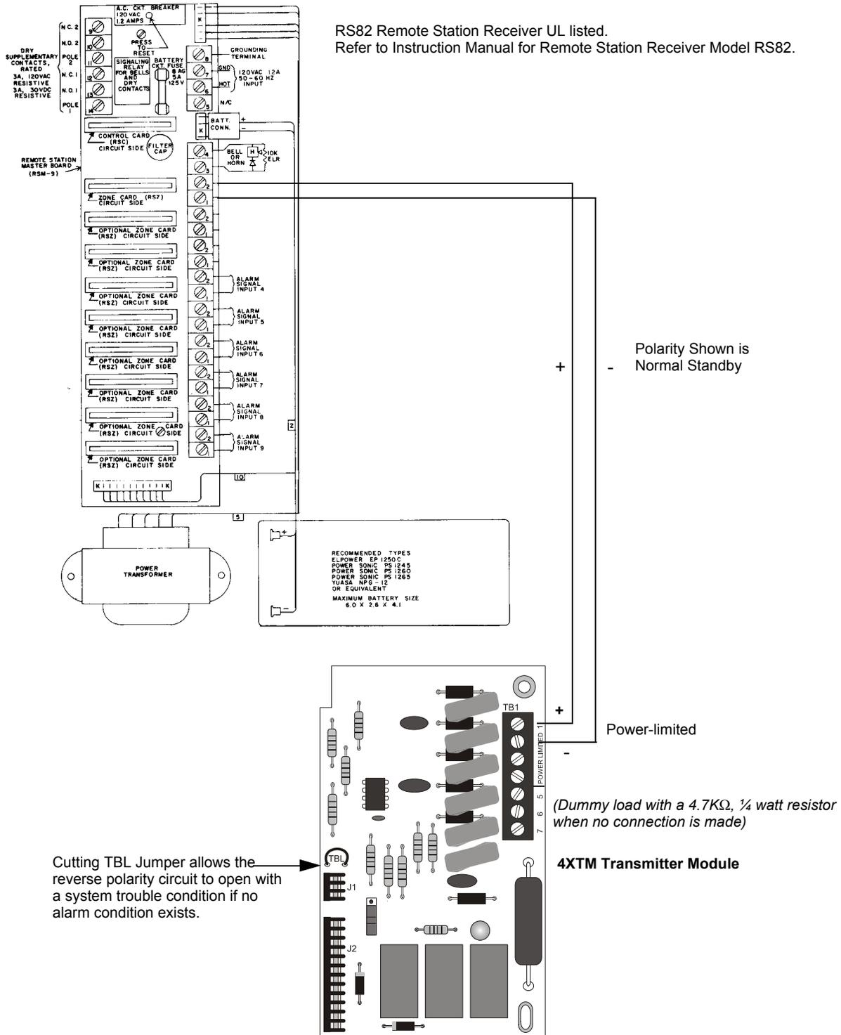
Figure B.3 Remote Station Connection Using 4XTM Module
