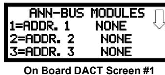
Pressing the down arrow key will allow the programmer to view additional screens displaying Addresses 1 - 8. Pressing the number corresponding to the desired address will display a screen with technical information about the selected module.
