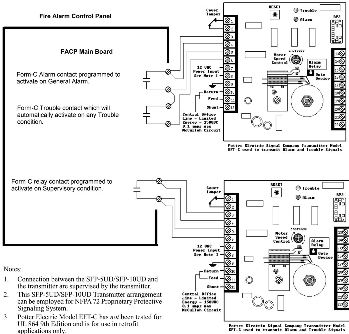
Figure B.4 Proprietary Protective Signaling System
