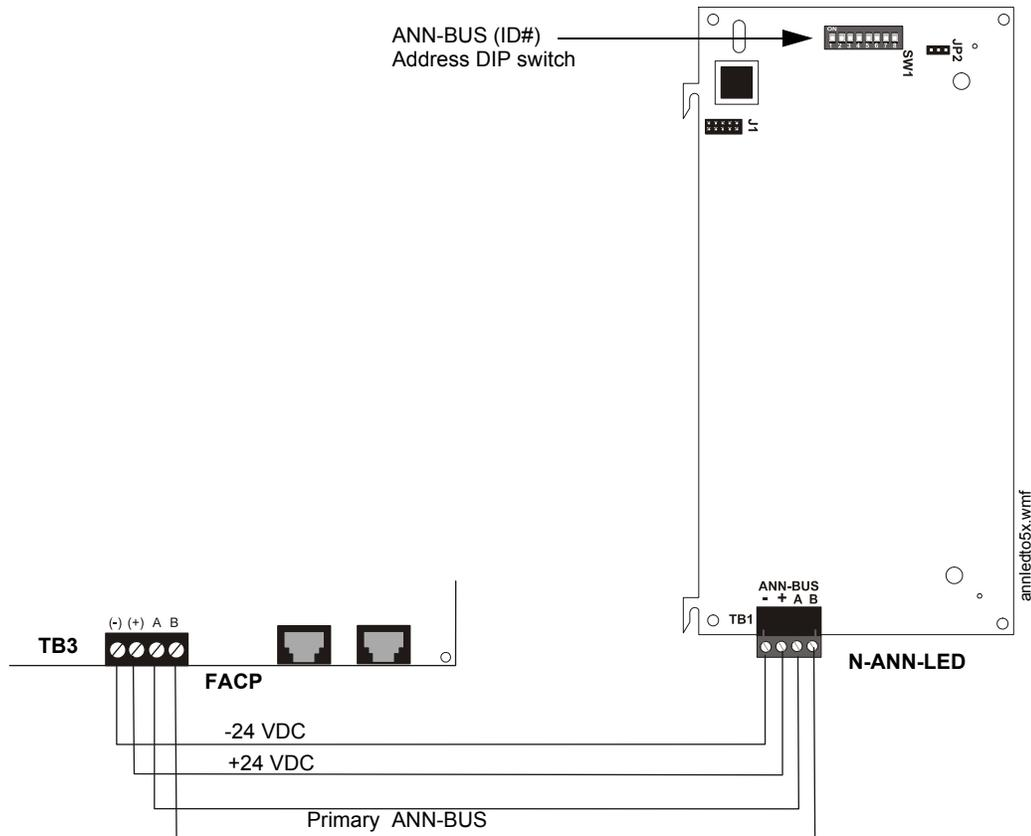
Figure 2.27 N-ANN-LED Board Layout and Connection to FACP
