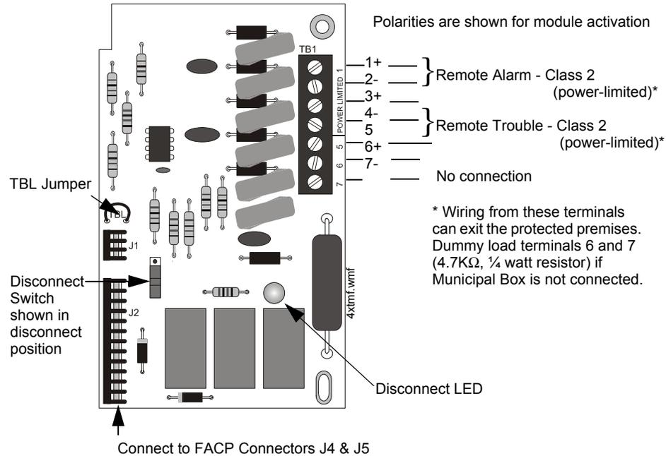
Figure 2.17 4XTM Transmitter Module
